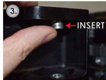
Reinstall the the drive roll and gear assembly into the bail. Take care to ensure the insert (left) and the bearing (right) are inserted prior to inserting the bolt.
