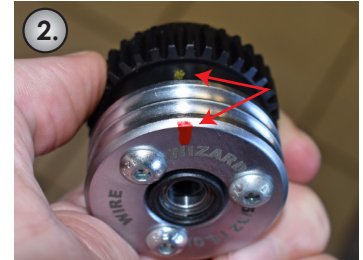
Install second drive roll and use a marker to mark the drive roll, in line with the yellow mark on the gear.
